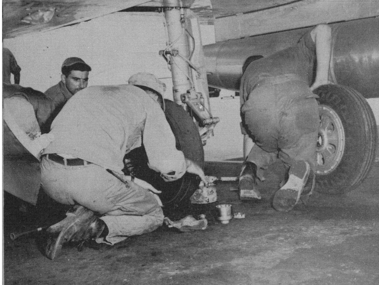
Maintainers replacing tires on 95 FIS F-86D (USAF photo)
